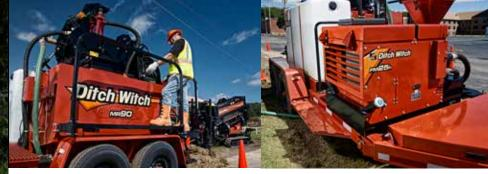
By reclaiming, recycling and reusing drilling mud, you retain profits that others are literally throwing away. You'll profit even more with the Ditch Witch® MR90, the most advanced, most productive mud recycler on the market. The MR90 can mix and recycle drilling mud as well as handle spoils, for exceptionally costeffective production. Among its many exclusively cost-efficient features: It has the fastest setup time on the market and it's the only mud recycler you can transport full of fluid.
