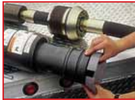
Wear rings increase tool performance and durability.
