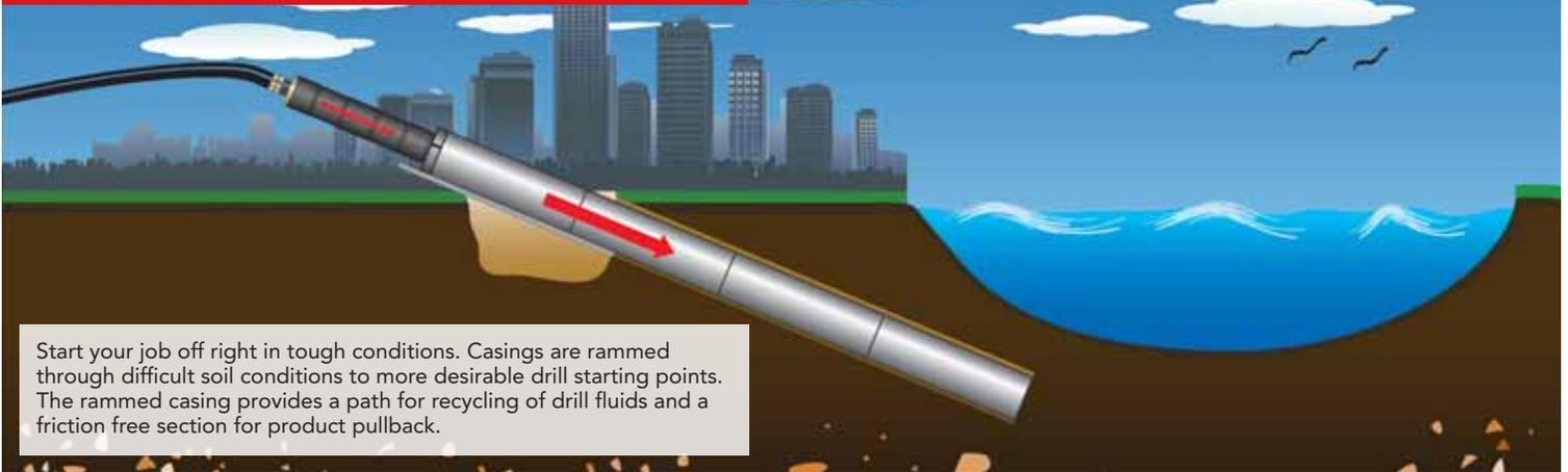
Start your job off right in tough conditions. Casings are rammed through difficult soil conditions to more desirable drill starting points. The rammed casing provides a path for recycling of drill fluids and a friction free section for product pullback.
