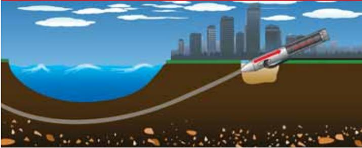
Recover your expensive, stuck drill stems! Attach the rammer to the drill stem with a fabricated adapter. The impact force of the rammer combined with static pullback is used to extract stuck drill stems.
