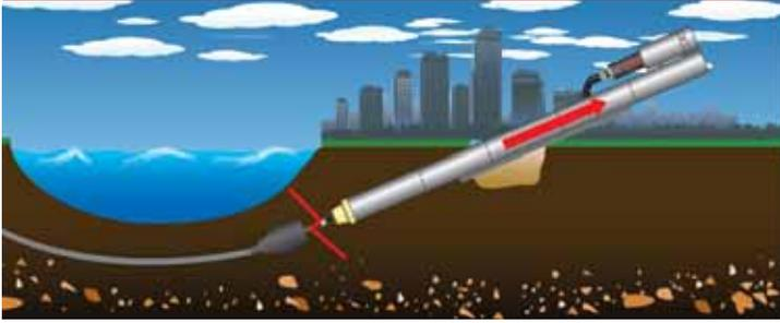
Recover your product pipe using the extraction method. The impact force of the rammer is combined with static pullback to extract product pipe so you can save expensive pipe and bore again.
