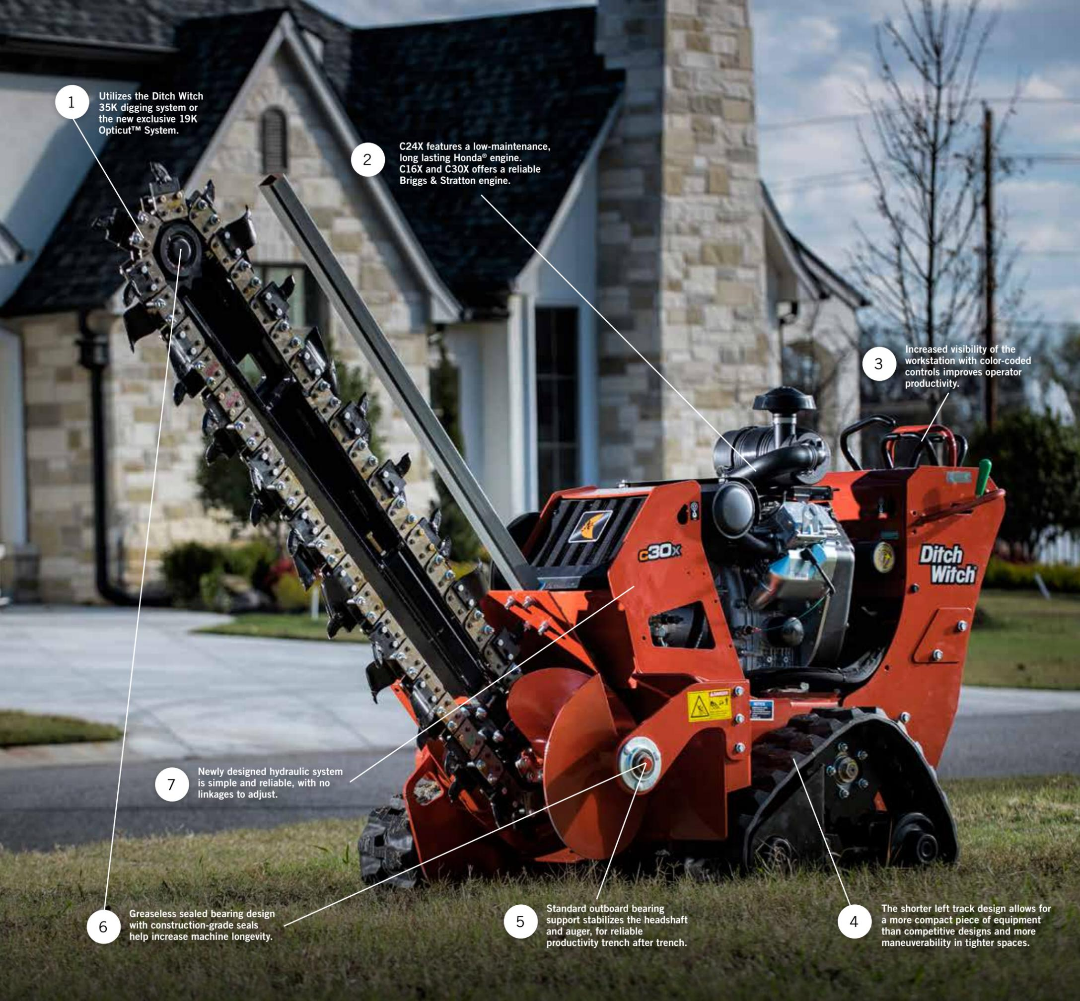
1 Utilizes the Ditch Witch 35K digging system or the new exclusive 19K Opticut™ System.
