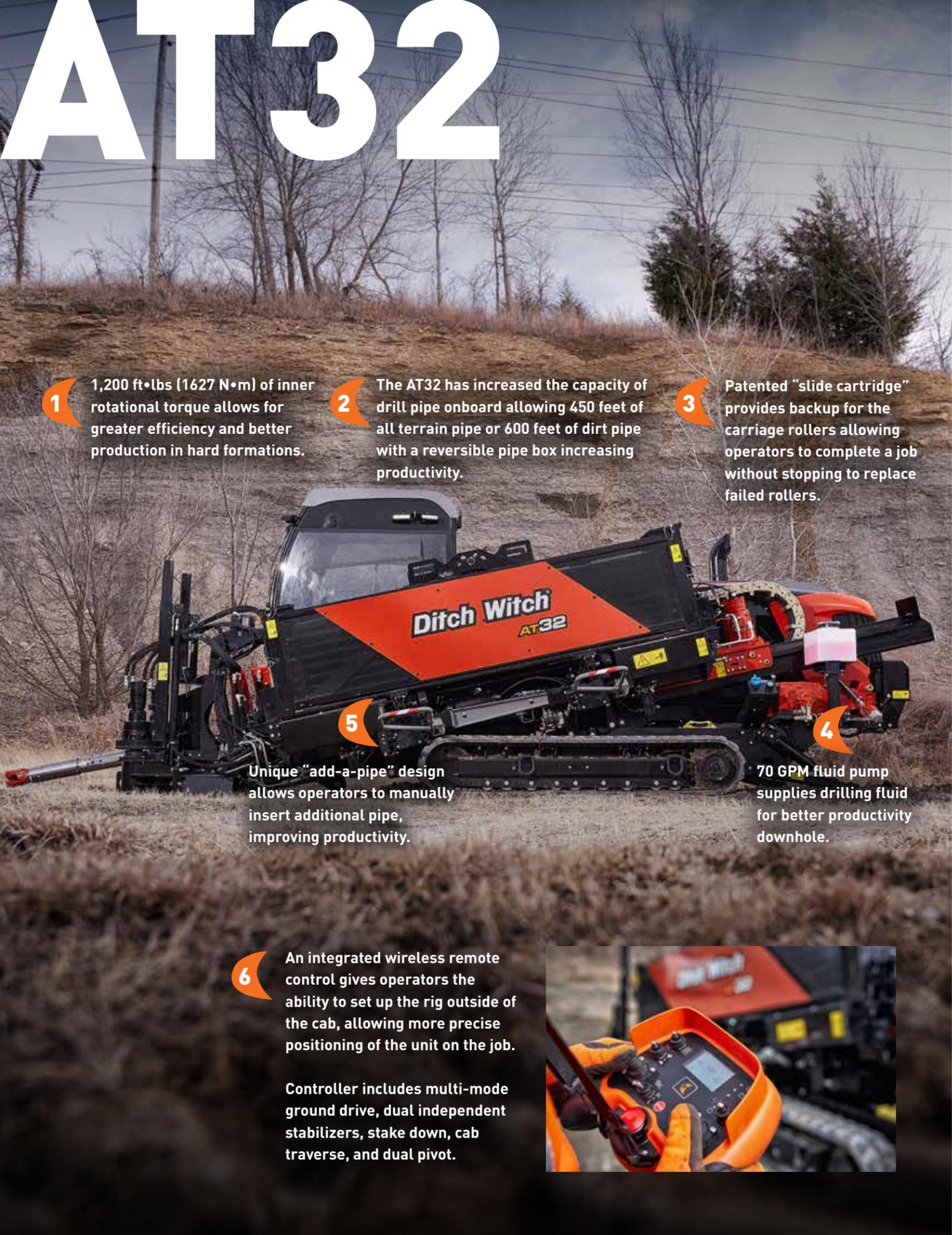
**1** 1,200 ft•lbs (1627 N•m) of inner rotational torque allows for greater efficiency and better production in hard formations.
